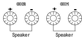
These are suitable for banana plugs, spade lugs or bare wires. Spade lugs and bare wires should both be screwed down tightly to exclude oxygen, and care should be taken to avoid loose strands of wire that may cause short circuits.
