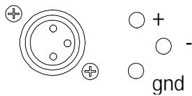
These type of jacks feature on much audio equipment and are convenient if the amp is frequently connected and disconnected, such as for mobile set-up. The plugs used should wired as per
