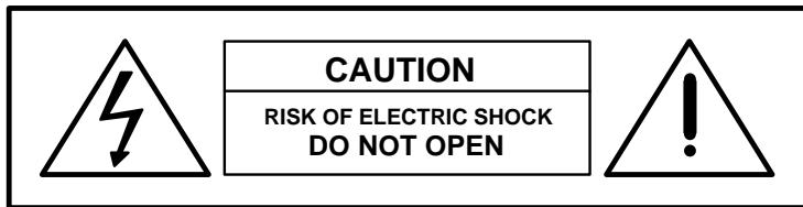
The lightning flash with arrowhead symbol, within an equilateral triangle, is intended to alert the user to the presence of uninsulated "dangerous voltage" within the product's enclosure that may be of sufficient magnitude to constitute a risk of electric shock.
